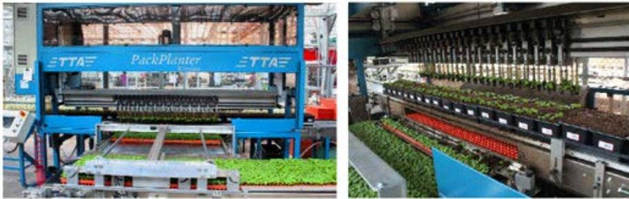
*Left: TTA's Wireless PackPlanter is the newest—and fastest—of Metrolina Greenhouses' current stable of transplanters. Right: Wireless servo grippers pick up one line of 48 plugs, then separate into two lines of 24 for planting, resulting in high speed with smooth movement.*
